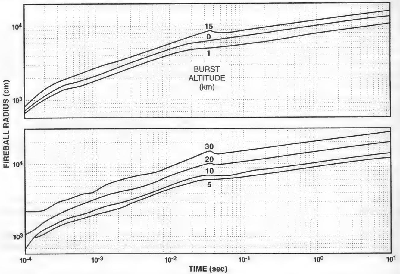
Figure 6.2. Fireball Radius Versus Time Curves for a 1-KT Burst at Various Altitudes.
